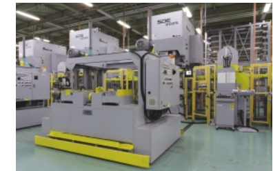
The presses process workpieces while automatically switching among more than ten types of molds. This intelligent equipment is a vital component of variable-model/variable-volume production.
