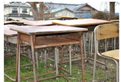
Even after being washed, desks and chairs which have once been immersed in seawater will eventually rust.
