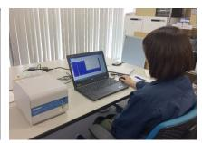
Scanning for heavy metals using X-ray fluorescence
